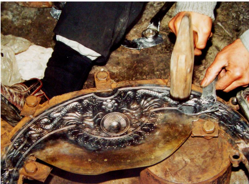
Design made by hammering (repoussé) the raw metal foil into the mould: 'Silver smith', Kaili Market, Guizhou Province
